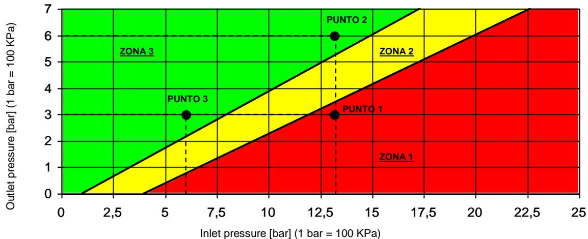
In order to avoid cavitation phenomena and therefore excessive component noise, we recommend choosing the number of pressure reducing valves necessary for a determinate pressure differential, according to the information in the "CAVITATION DIAGRAM". The cavitation diagram shows the three operating zones of the pressure reducing valve in function to the inlet and outlet pressures:
