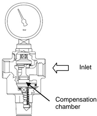
When the uses to be served are closed, the downstream pressure increases, pushing the reducer piston downwards. In this way, the shutter closes the passage section of the reducer maintaining the setting value set on the spring constant; in fact, the minimum pressure difference across the shutter permits the perfect closing of this latter.
