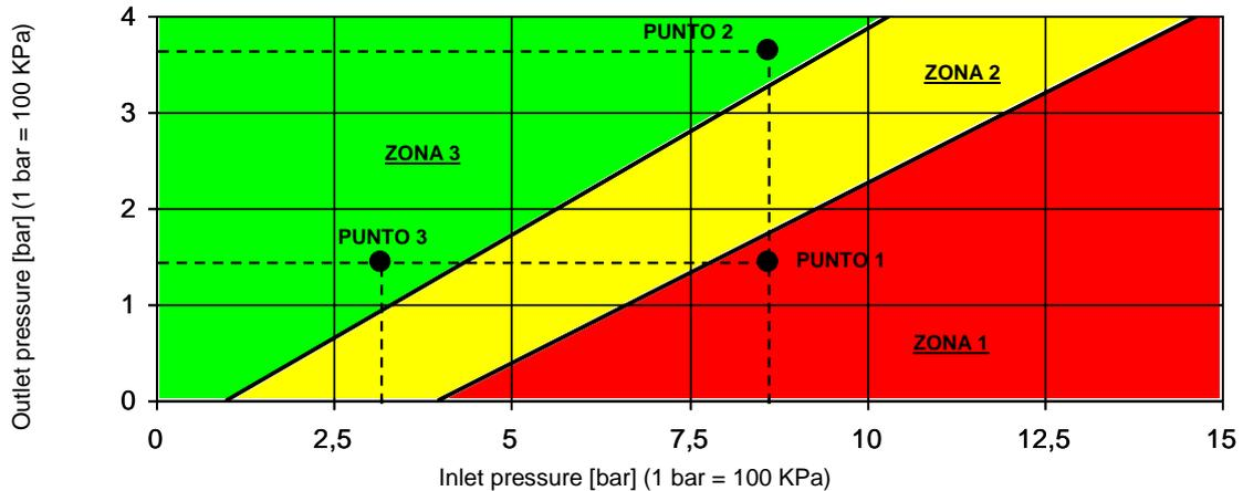
In order to avoid cavitation phenomena and therefore excessive component noise, we recommend choosing the number of pressure reducing valves necessary for a determinate pressure differential, according to the information in the "CAVITATION DIAGRAM". The cavitation diagram shows the three operating zones of the pressure reducing valve in function to the inlet and outlet pressures:
