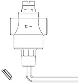
The final calibration of the pressure reducing valve must be performed with the hydraulic circuit completely full and with all the uses closed, otherwise false values would be obtained owing to the fact that the downstream pressure reduces in relation to the necessary flow rate, during any supply.
