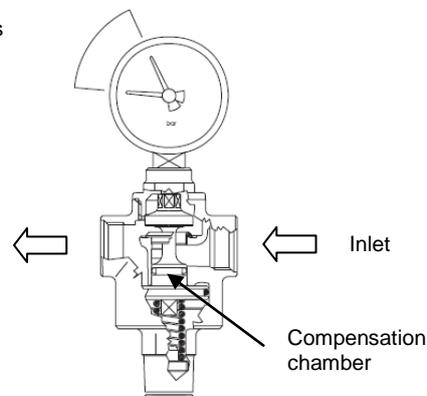
When the uses are opened downstream, the pressure exerted on the piston is lessened in favour of the force exerted by the spring on the shutter permitting it to open with the constant passage of the fluid. As the water demand from the user network increases the pressure on the piston decreases and more water passes.
